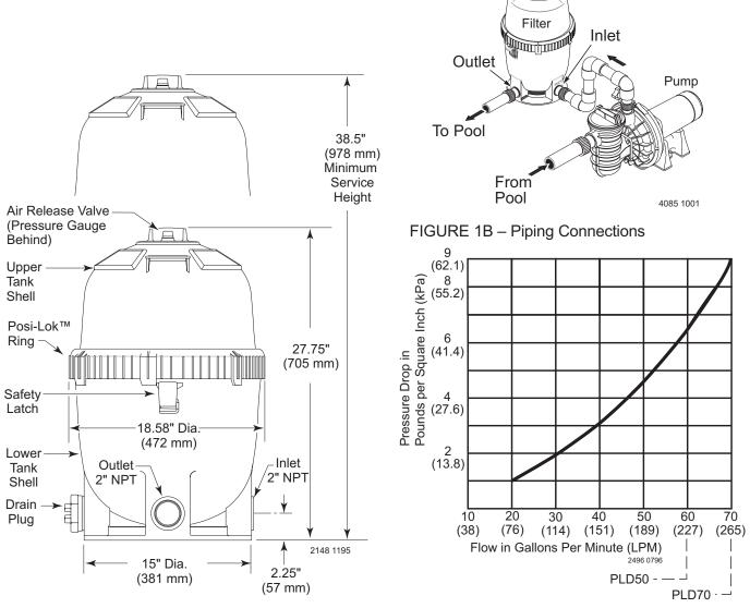
FIGURE 1A – Dimensions in inches (mm)
