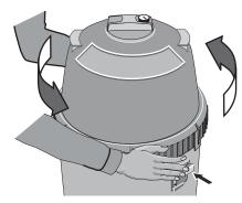
Figure 4 – Depress safety latch to unscrew Posi-Lok™ Ring.
