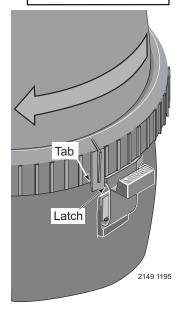
Figure 3 – Rotate Posi-Lok™ Ring until tab locks behind the safety latch.
